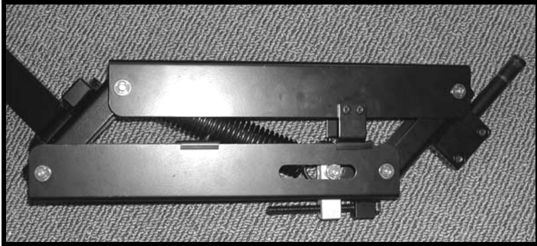
The Glidecam® V-8 with a single spring across it's diagonal (courtesy of Taylor)
